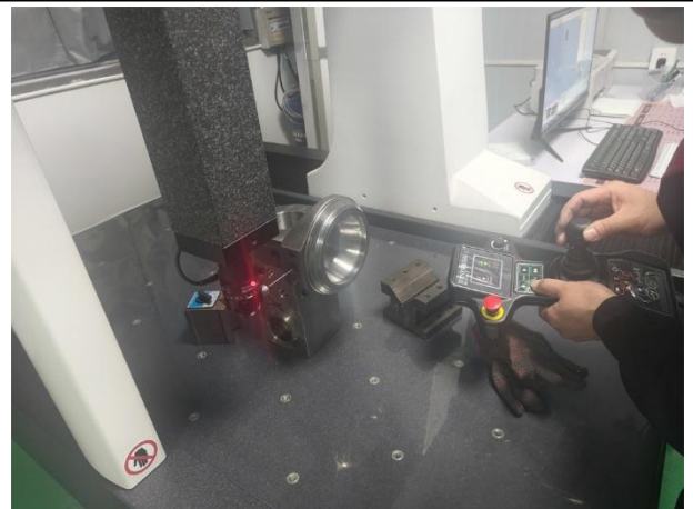
Measuring: CMM testing
