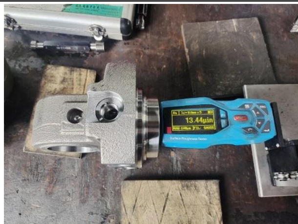
Measuring: Ra 63 testing
