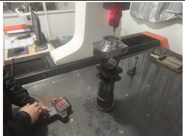
Measuring: CMM testing
