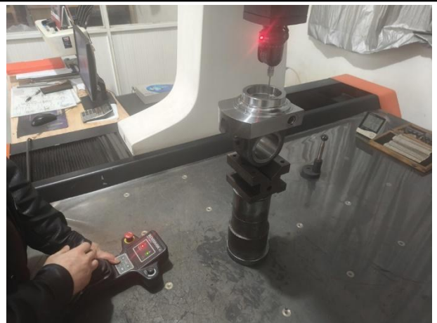
Measuring: CMM testing
