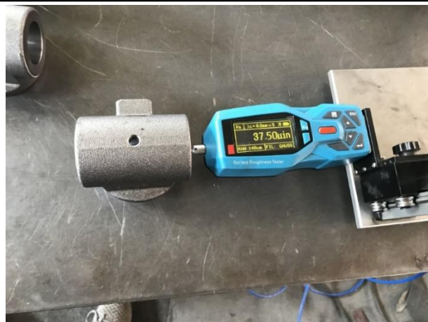
Measuring: Ra63 testing
