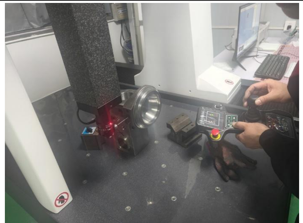
Measuring: CMM testing
