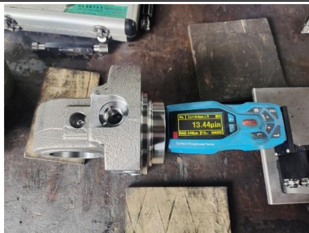
Measuring: Ra 63 testing
