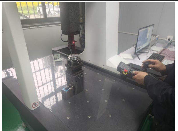
Measuring: CMM testing
